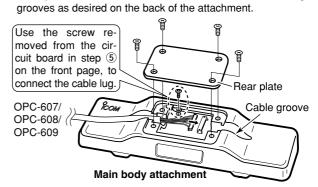
④ Connect the supplied flat cable\* and ground cable (coming from the RMK-3) as shown below.
