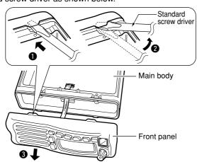
4 Disconnect the flat cable from the front panel.
